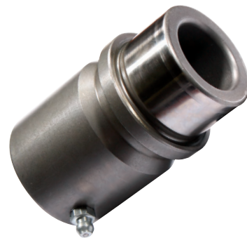
Guide Bush, Thick & Long Type (for heavy dies / with collar & lubricating)
