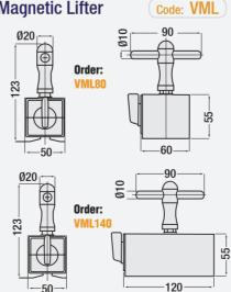
Carrying Capacity: VML.80 (80 Kg) / VML.140 (140 Kg). Unit Weight: VML.80 (1.2 Kg) / VML.140 (2.2 Kg). It holds work pieces easily and elastically and is a useful carrying product.
